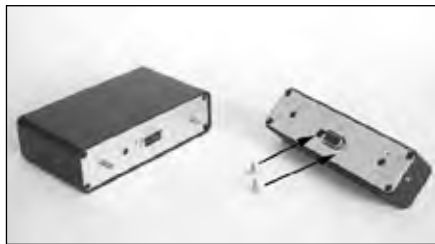
Figure 1.1b To connect the separated unit, first insert the standoffs to secure the cable connectors.
