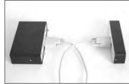
Figure 1.1c Secure the connecting cable by fastening the thumbscrews into the standoffs.
