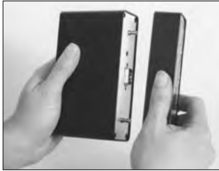
Figure 1.1a Separating the computer/display unit.
